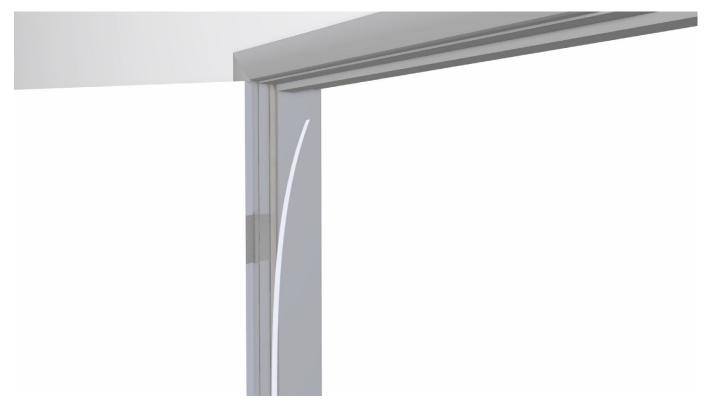
**Step 3:** On the top of the door, measure for the width of the seal.
