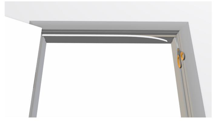
**Step 4:** Repeat Step 3 for the handle side of the door. Measure for the height of the seal.
