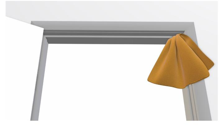
**Step 2:** On the hinge side of the door, measure for the height of the seal.
